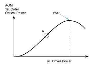
As can be seen from the curve above, applying RF power in excess of Psat will cause a <u>decrease</u> in first order intensity (a false indication of insufficient RF power)
