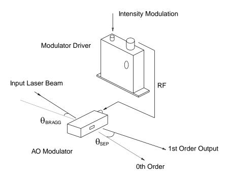
The input Bragg angle, relative to a normal to the optical surface and in the plane of deflection, is given by:
