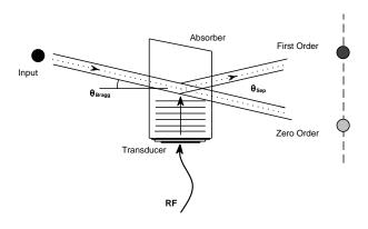
Diffraction Efficiency (DE) =  $\frac{\text{First order (RF On)}}{\text{Zero order (RF Off)}}$
