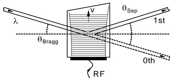
An AO device works through the interaction of sound (RF) and light. This is achieved via a piezo-electric transducer bonded to one face of a suitable crystalline material. When an RF drive signal is applied to the transducer, a travelling acoustic wave is produced in the crystal. This creates areas of compression and rarefaction, similar to the slits in a diffraction grating.
